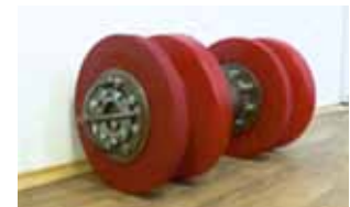
Cup-disk cleaning pig "VOSTOK-M4" with "VOSTOK-VR" installed in the front, prior to the trial.
